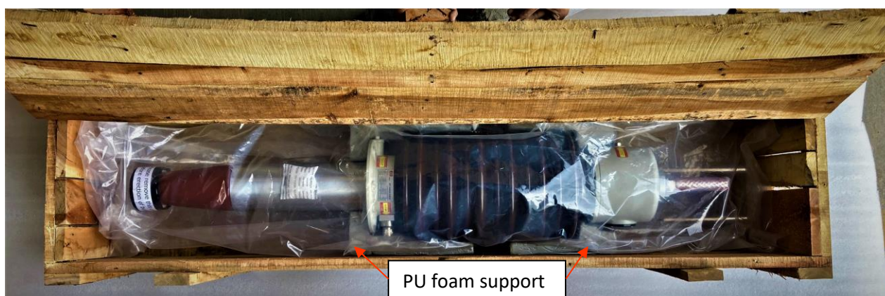
Figure 1.2: Bushing packed with polythene bag cover and Bottom PU foam support
